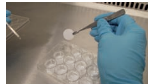
Figure 3. Alvetex® discs can easily be removed from the 12-well plate using flat ended forceps (Fisher Scientific, MNK-155-M).
