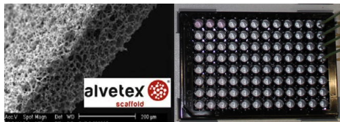
Figure 1 Left: SEM of the Alvetex Scaffold made from polystyrene. Average void size 40 \mu\text{m} . Right: photograph of an Alvetex Scaffold 96-well plate in SBS format with four fixed tips from a Freedom EVO Liquid Handling (LiHa) Arm
