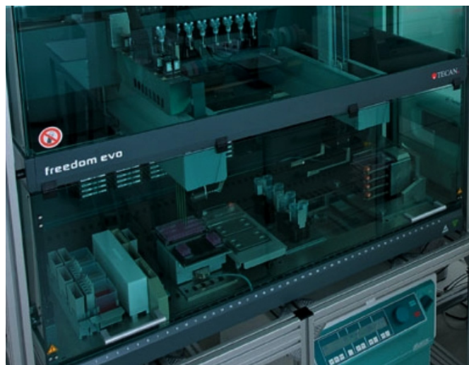
Figure 2 The Freedom EVO cell biology workstation
